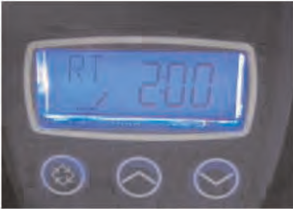
Fig 3 Ecosmarte® Control Valve is displaying the time set for backwash (02.00AM). Backwash starts automatically when the preset usage has been reached, at 2.00AM when total gallons have been used that day.
